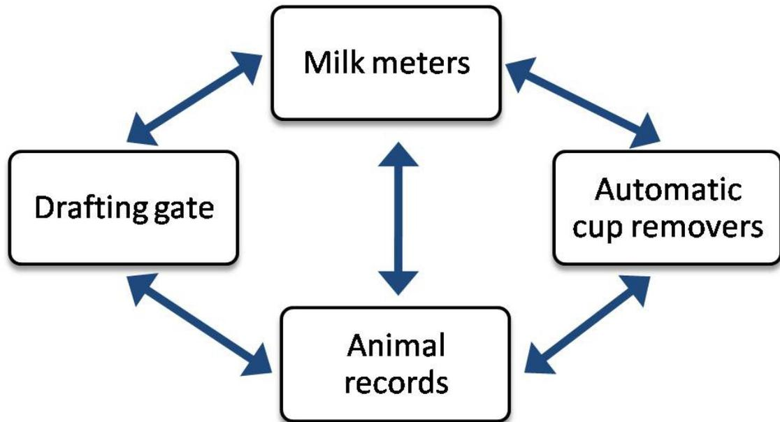
**Figure 2.** Mapping out relationships between different components can be used as a design tool or aid for purchasing decisions. The diagram illustrates our ideal integration of different cowshed components, we chose technology that was able to integrate in the way shown. Different farms will have different scenarios.
